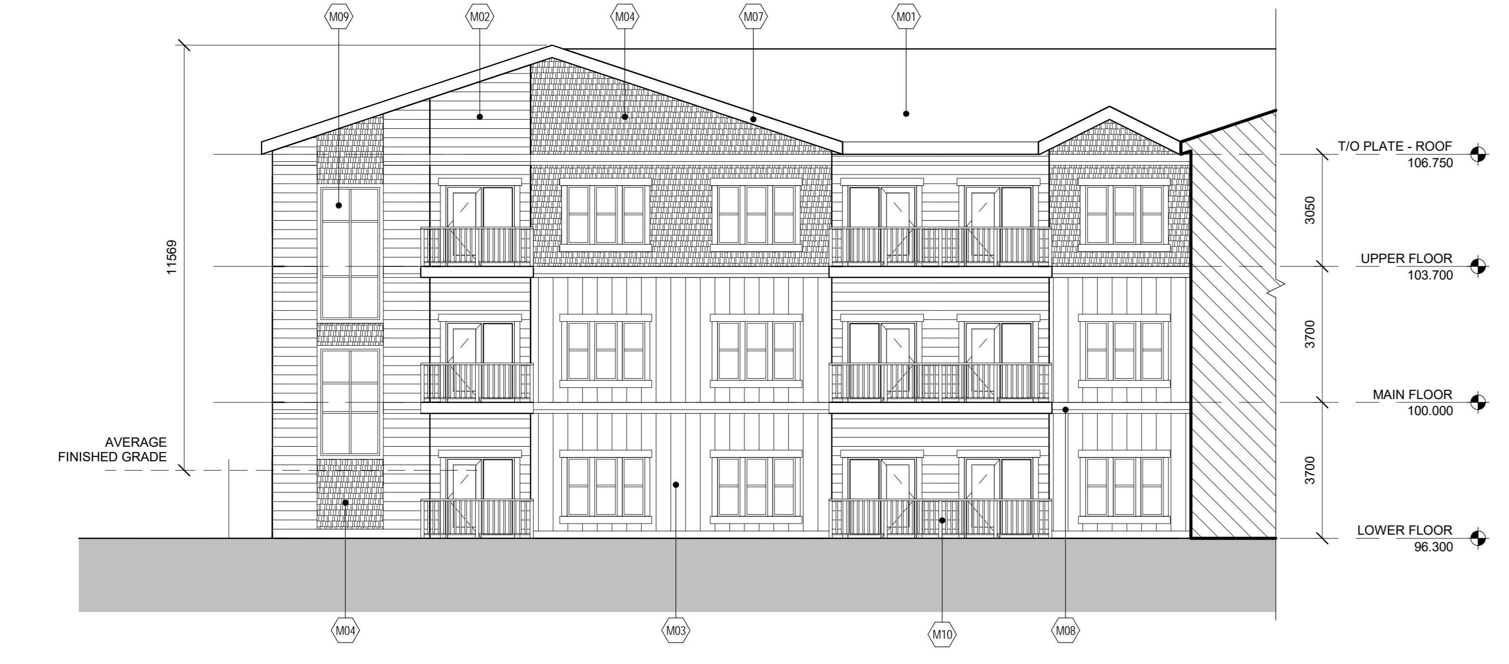
7 HOUSE B - WEST ELEVATION DP-201 1:100
