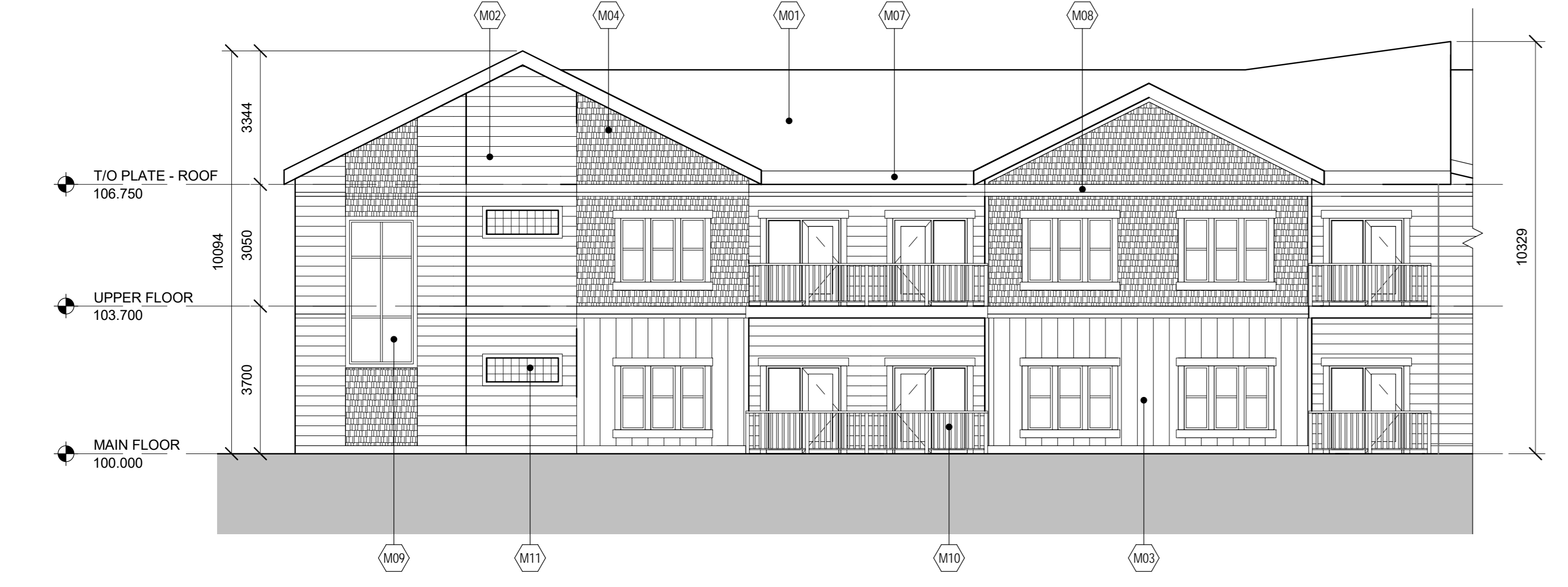
3 HOUSE A - WEST ELEVATION DP-201 1:100
