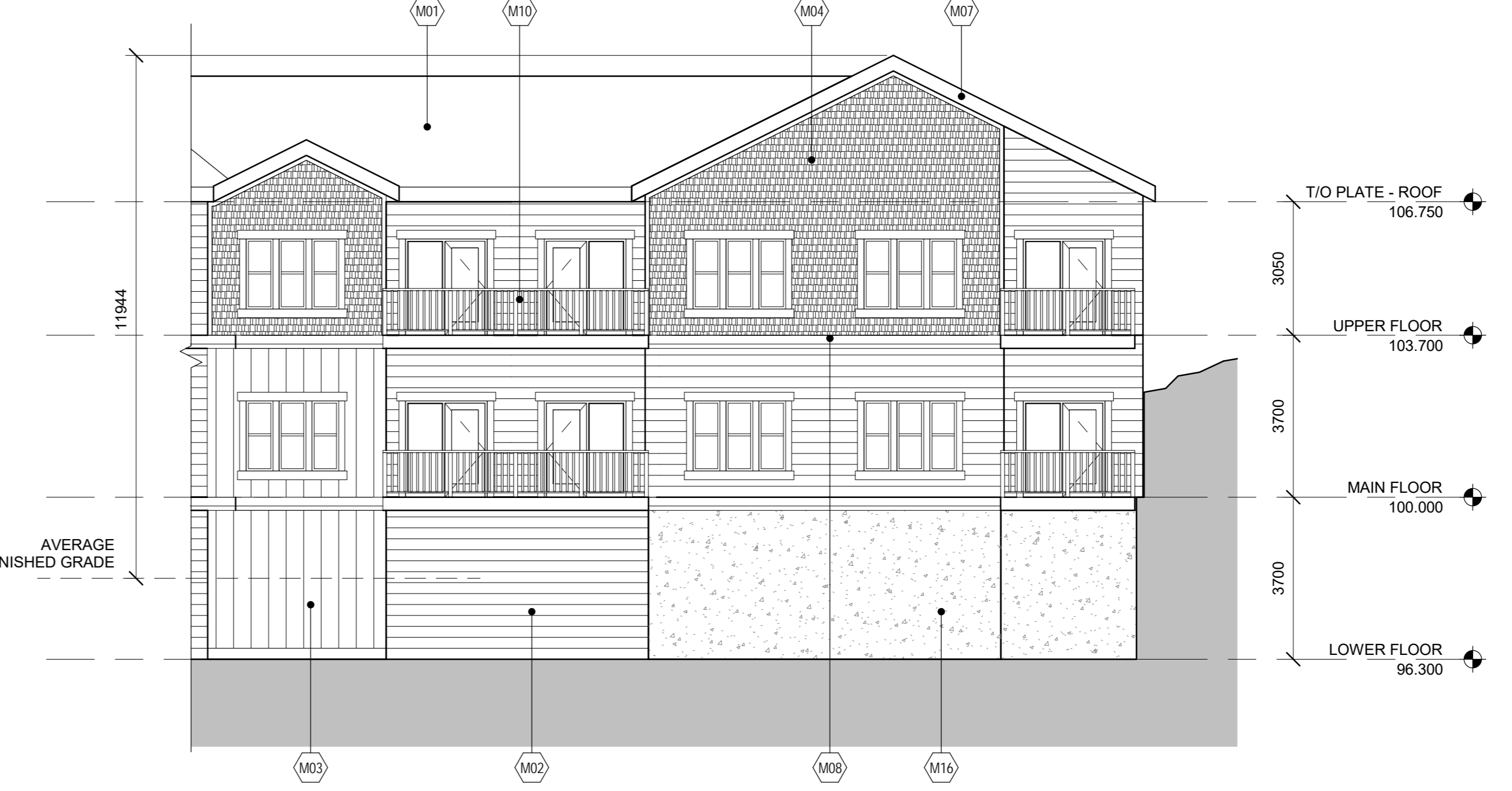
6 HOUSE A - EAST ELEVATION DP-201 1:100
