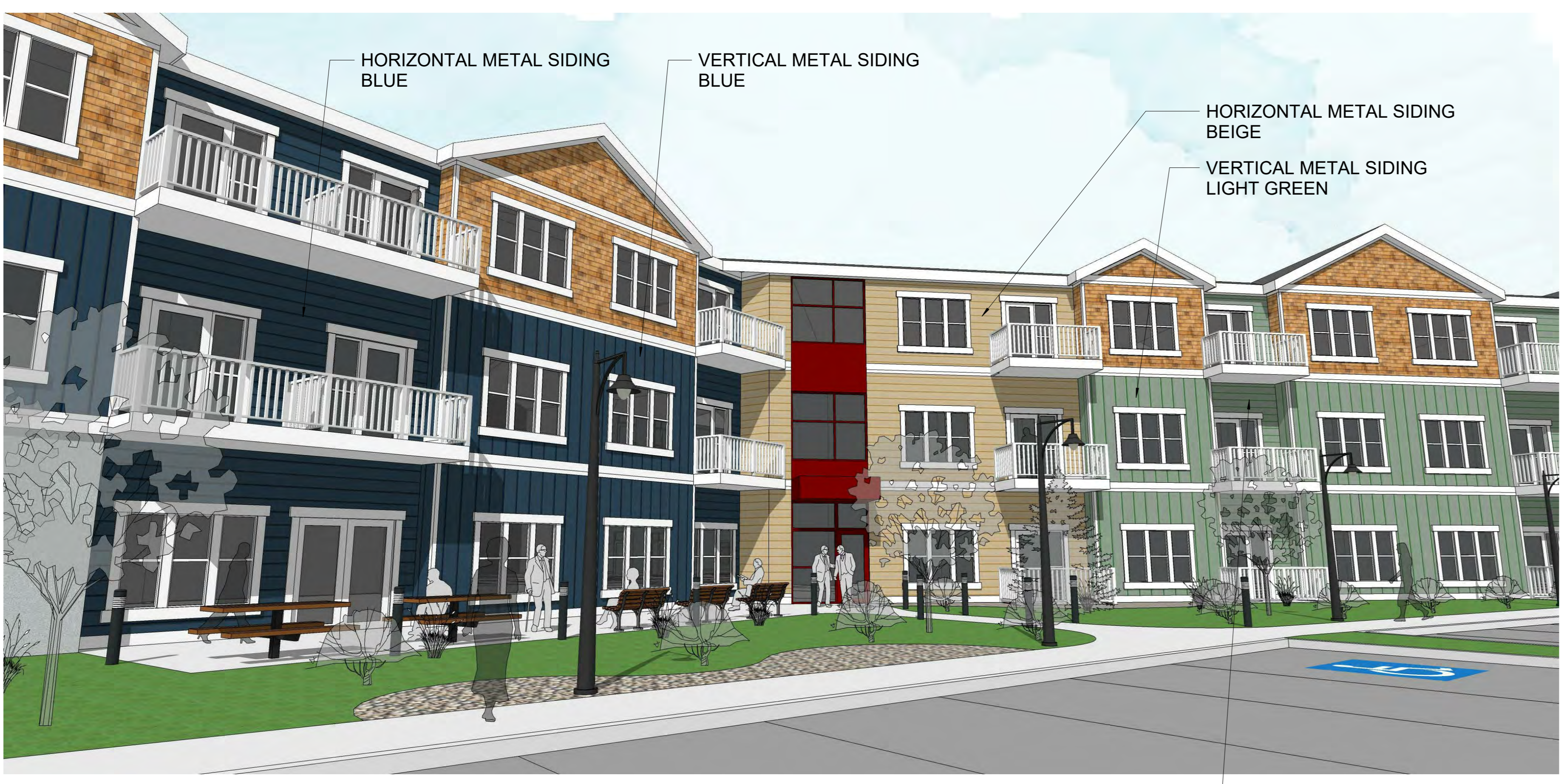
SECOND ENTRANCE HORIZONTAL METAL SIDING LIGHT GREEN VERTICAL METAL SIDING BLUE HORIZONTAL METAL SIDING BEIGE VERTICAL METAL SIDING LIGHT GREEN HORIZONTAL METAL SIDING BLUE
