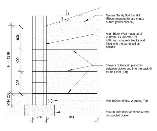
All above dimensions are based on initial design assumptions, and all are minimum required amounts. When the wall is entirely vertical, a minimum of 3 layers of Geogrid is necessary to provide lateral stability and connection for the blocks. Please, refer to manufacturers' manuals for Allan blocks and Geogrid for details and application instructions.
