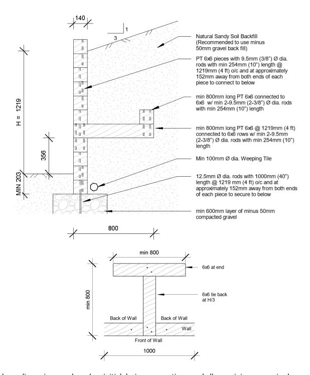
All above dimensions are based on initial design assumptions, and all are minimum required amounts.
