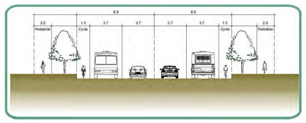
Exhibit 11-11: Highway 4 – Example of a Typical Cross-Section
