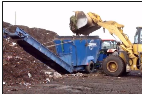
FIGURE 4 PTO MIXER USED AT CITY OF WHITEHORSE COMPOSTING FACILITY (SOURCE: TRANSFORM COMPOST SYSTEMS)
