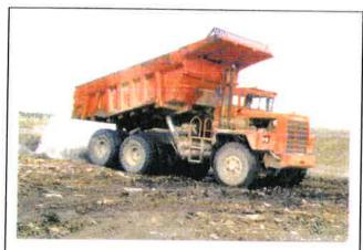
Photo 8-8 Deploying Water at Vancouver Landfill, 3,000 Gallons Per Load
