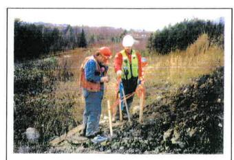
Photo 9-7 Measuring Gas Composition with Bar Hole
