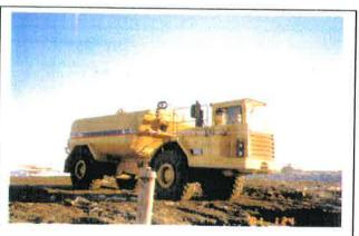
Photo 8-9 Water Truck Injecting Into Stinger
