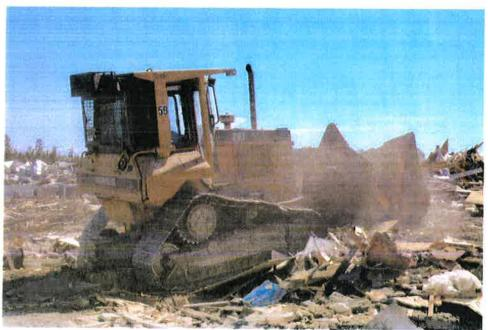
Photo 11-2 Bulldozer Compacting C&D Waste
