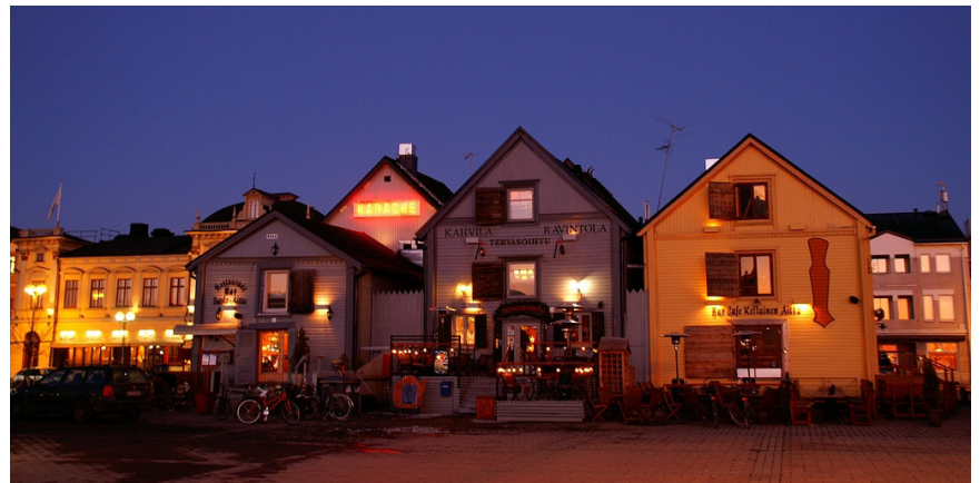
The lighting for this building follows Dark Sky principles. Relevant areas are lit with downcast lighting and no glare is created.
