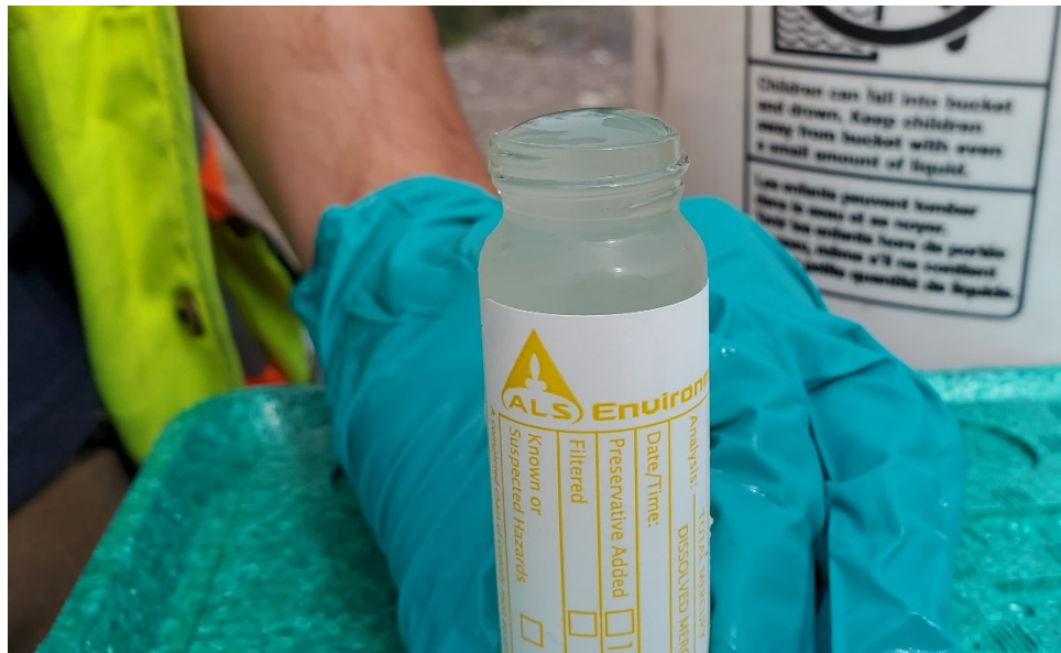
Figure 7: Meniscus of water in bottle before putting lid on
