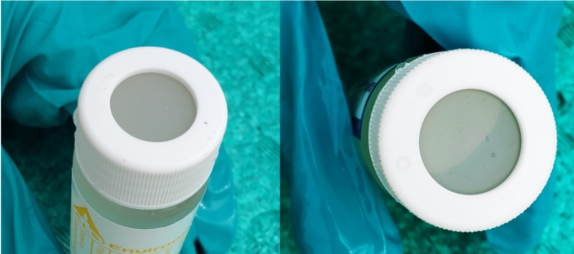
Figure 8: Bottle lid showing proper closure with no bubbles, and improper closure with an air bubble
