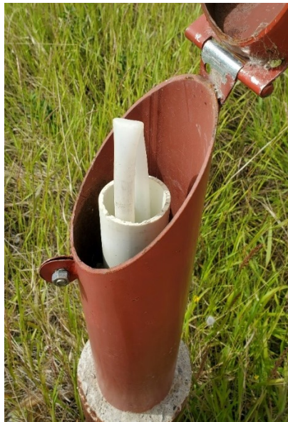
Figure 16: Tubing stored in well
