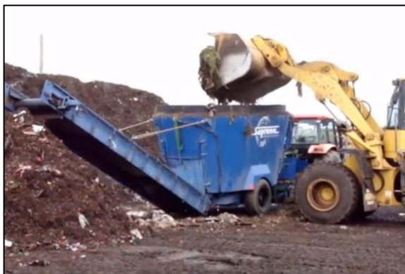
Figure 80: PTO Mixer used at City of Whitehorse composting facility
