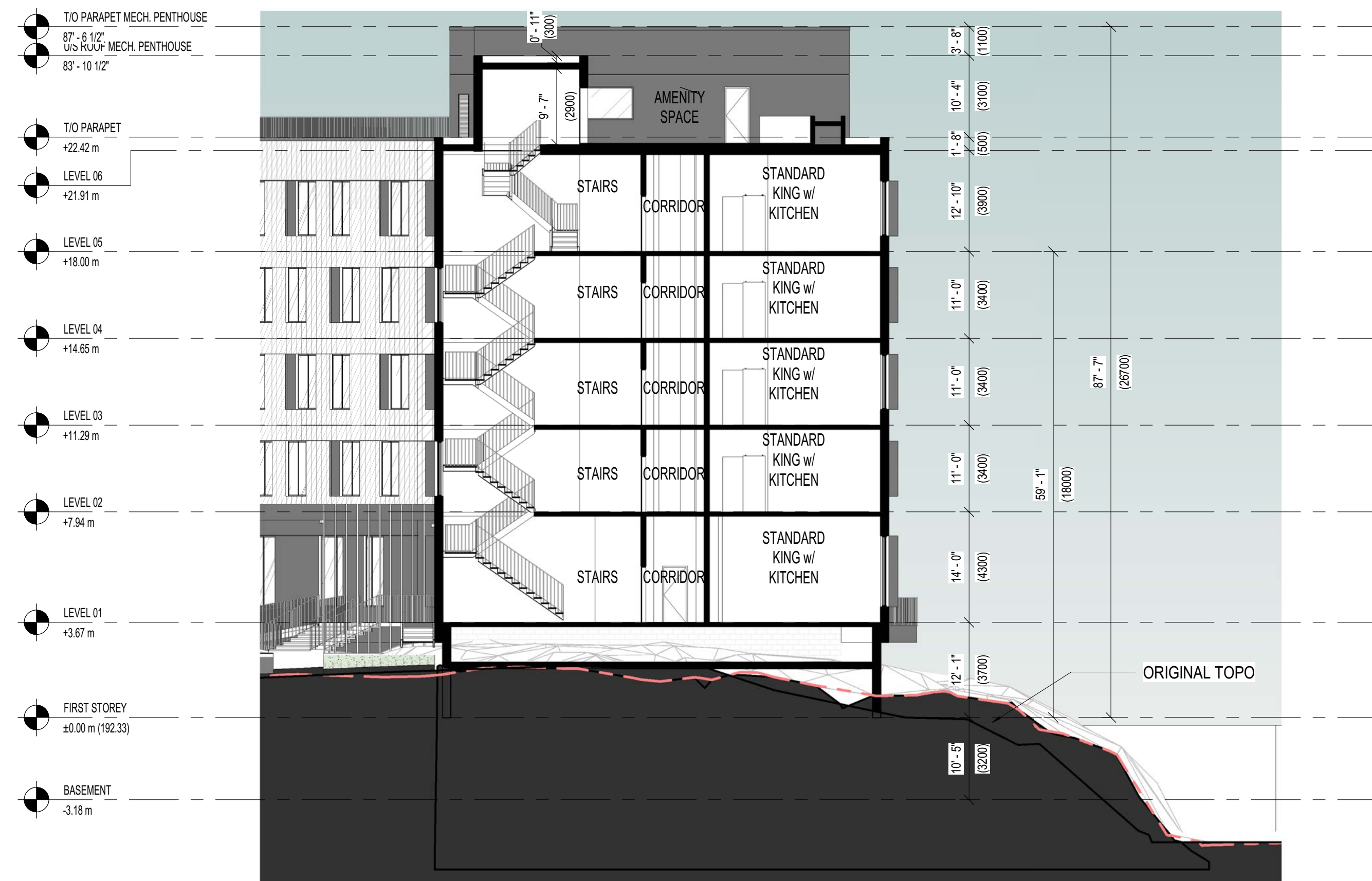
3 E-W SECTION THROUGH SOUTH EXIT STAIR DP-13 1:150
