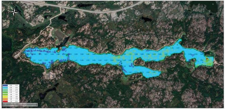
Figure 2 Fiddlers Lagona sludge thicknesses (m)
