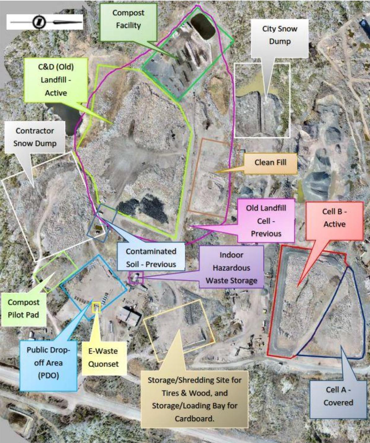
Figure 1: Solid Waste Facility Site Layout
