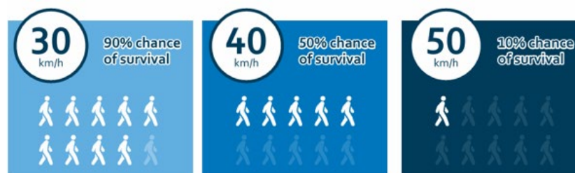
APPENDIX B FIGURE 3: RELATIONSHIP BETWEEN MOTOR VEHICLE SPEEDS AND PEDESTRIAN FATALITY RISK IN A COLLISION (Source: City of Kelowna, Safe Mobility Action Plan , 2024)
